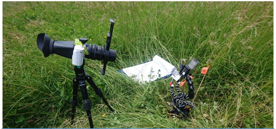
Plate 5: experimental set-up for obtaining UV and visual photographs
